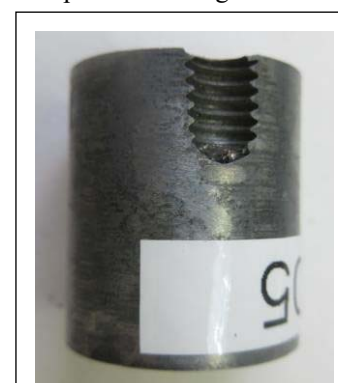
Fig. 6 Female thread for insertion piece mounting
