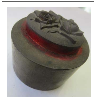
Fig. 9 Pattern integrated with the base plate
