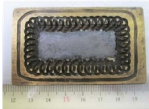
Fig. 6: Example of partially filled cavity with lead
