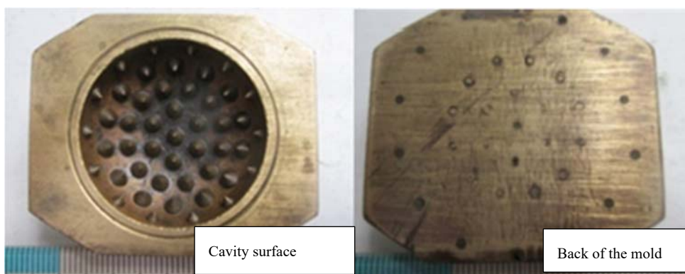
Fig. 4: Broaching base mold
